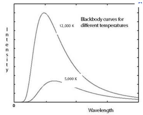
Identify and account for two differences in the curves. In what ways are they similar? Both peak at particular wavelengths, but the wavelengths are different. The higher temp gives off more light so its curve is bigger
